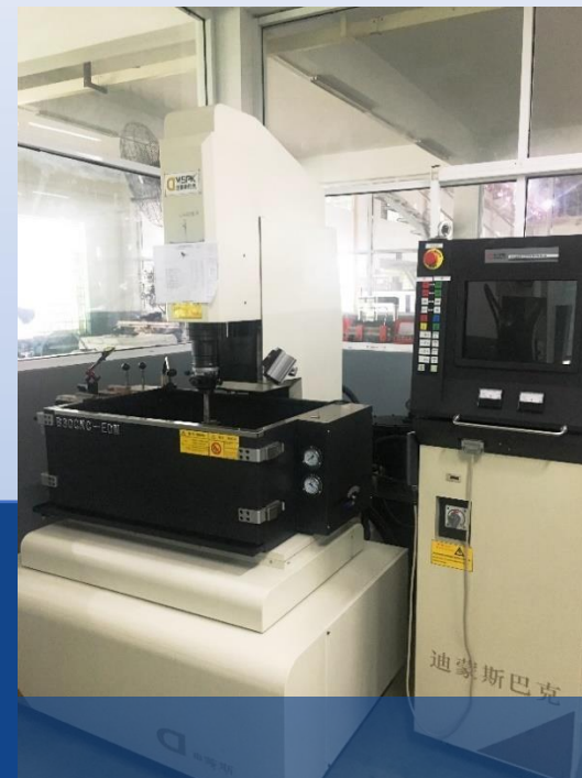
03 EDM (Electrical Discharge Machining)
