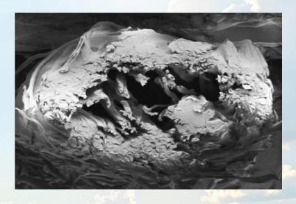
Upon dissolving Solucell, the yarn becomes hollow and is made of 100% cotton
